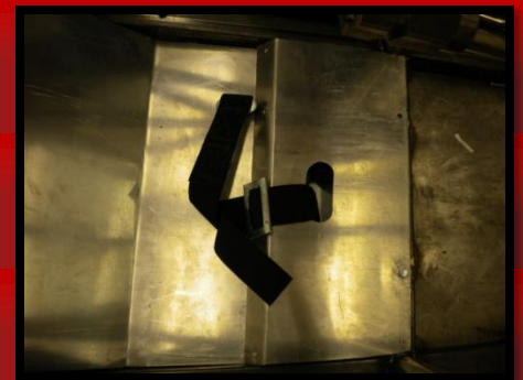
THE BOTTOM OF THE SEAT WHERE WE HAD TO CUT A HOLE FOR THE STRAP OF THE 5-POINT SAFETY HARNESS TO COME THROUGH.
