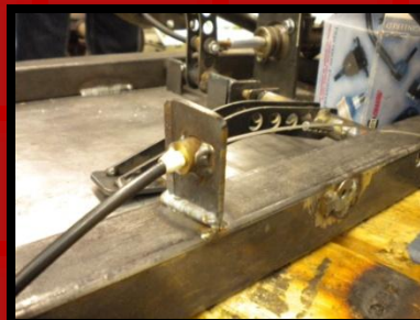
THE MOUNT THE HOLDS THE THROTTLE CABLE IN PLACE.
