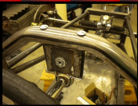
THE PLATE THAT WAS CREATED TO HOLD THE STARTER BUTTON.
